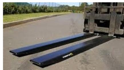
Why do extensions change the truck's capacity? This is because the farther you move the load's center of gravity (load center) forward, the more overturning moment you are creating. This is particularly evident in the event of a sudden stop.
