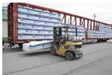
One situation that may require the use of multiple forklifts is loading a long unit of material (which is within your truck's capacity) on the top of a center beam rail car. Long materials sag which prevents you from fitting the load under the top center beam of the car.
